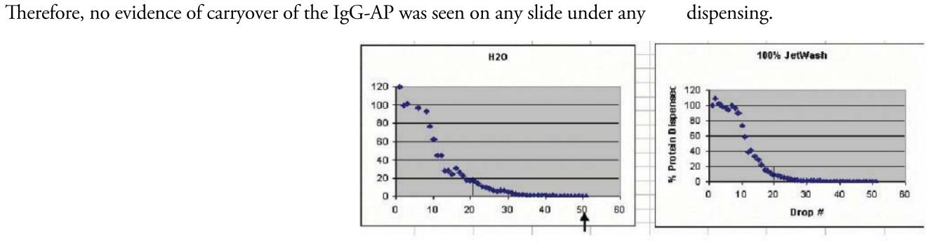
Efficient washing steps: Elimination of protein by various washing agents when compared to water. Water by itself is capable of washing protein from the system. Study performed on BioDot AD5000.
