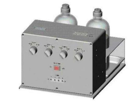
Flow-through vacuum degassing chamber with a single amorphous perfluorinated copolymer (Teflon<sup>®</sup> AF) degassing membrane. This compact design comprises continuously vented mini vacuum pump with a unitary PTFE diaphragm. Degassing efficiency is equal to fifty (50) times the degassing efficiency of other PTFE designs. Several vacuum degassing modules may be mounted in parallel on one arrayer. Eliminate any set-up time required for degassing prior to any dispensing experiment.
