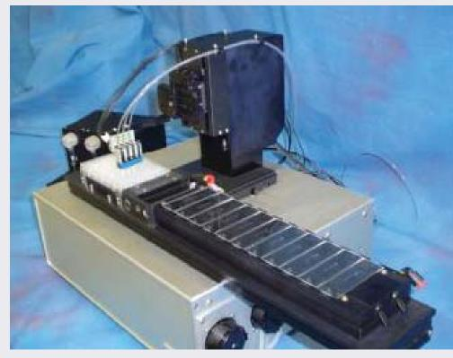
Scalability of dispensing channels for faster throughput: BioDot's arrayer equipped with one dispensing channel can print twenty microarrays in 6 min 14 seconds, each array being 8 x 12 dots. It would take 3 min 7 seconds to do the same spotting experiment with two dispensing channels (14 nL spots, 1.02 mm center-to-center distance, 18 mm spacing between arrays).
