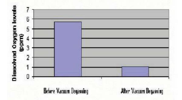
Efficiency of flow-through vacuum degassing chamber to lower the level of dissolved gas inside a fluid. Experiment performed with BioDot syringe pump. The fill flow rate is 30 uL /sec. The prime flow rate is 60 uL/sec. The vacuum efficiency is constant overtime and guarantees the degassing efficiency.
